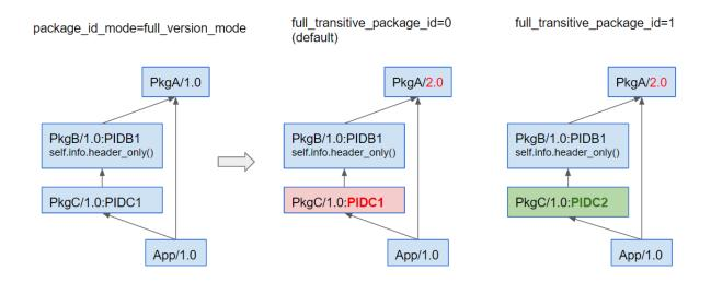
With the default behavior, the header only PkgB is isolating PkgC from the upstream changes effects. The package-id PIDC1 we get for PkgC/1.0 is exactly the same when depending on PkgA/1.0 and PkgA/2.0.
