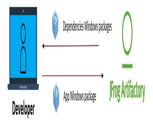
2. Packages can be cross-built for the target device using the Yocto SDK and uploaded to Artifactory, even automated in a CI process.
