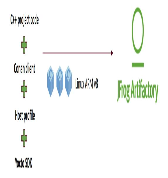
3. Once the cross-built packages are available in Artifactory, the application can be directly deployed to the Yocto image. This step can also be automated also in a CI. it from sources again.
