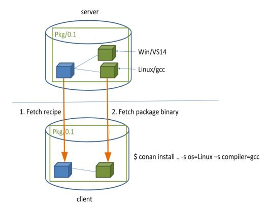
For example, the command **conan install .. --settings os="Linux" --settings compiler="gcc"**, performs these steps:
