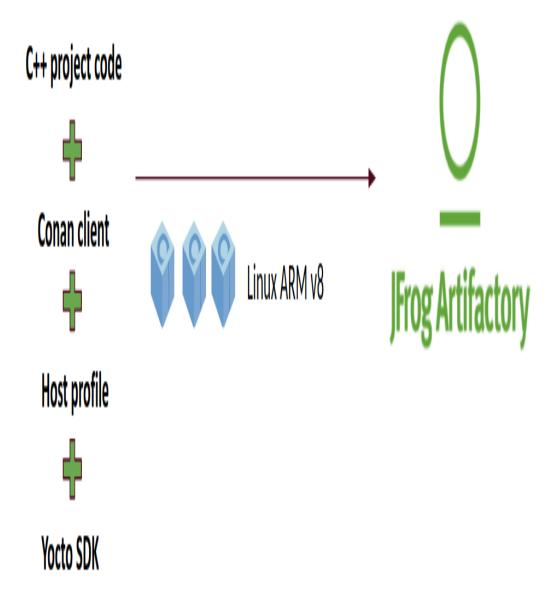
3. Once the cross-built packages are available in Artifactory, the application can be directly deployed to the Yocto image. This step can also be automated also in a CI. it from sources again.
