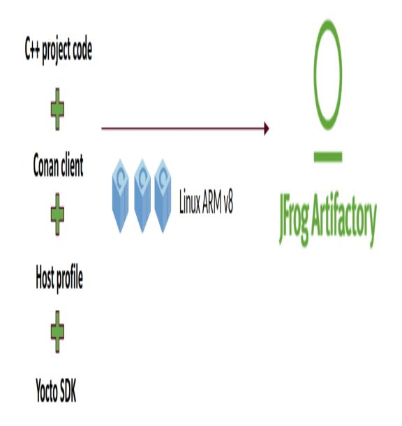
3. Once the cross-built packages are available in Artifactory, the application can be directly deployed to the Yocto image without building it from sources again.
