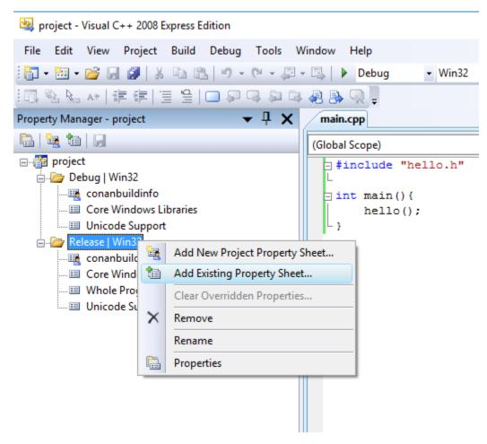
Note that for single-configuration packages (which is the most typical), Conan installs Debug and Release packages separately. So a different property sheet will be generated for each configuration. The process could be:
