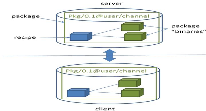
Installation of packages from servers is also very efficient. Only the necessary binaries for the current platform and configuration are downloaded, not all of them. If the compatible binary is not available, the package can be built from sources in the client too.
